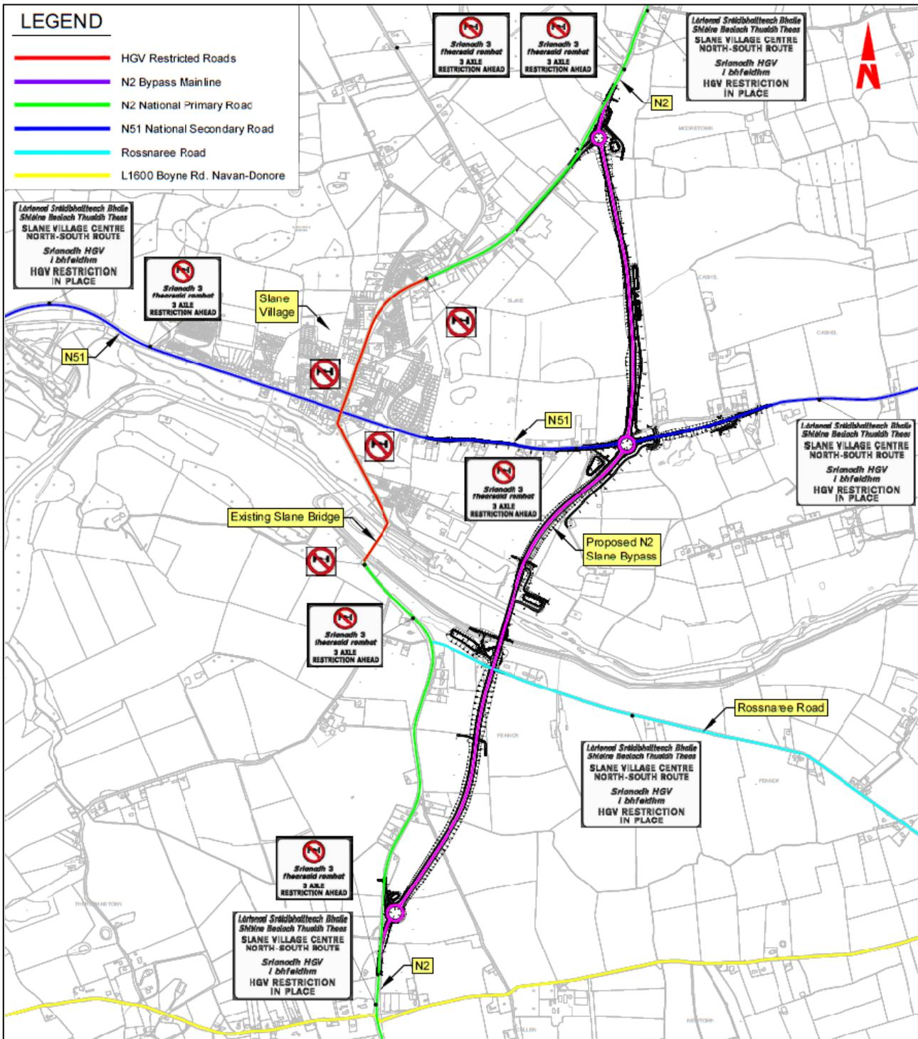
Figure 4.32: Illustrative Layout of implementation of a Proposed HGV Ban in Slane Village
