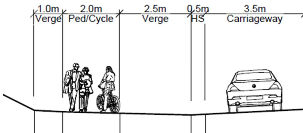
**Figure 4.6: Indicative Cross-Section showing Two-Way Cycle / Pedestrian Facility**
