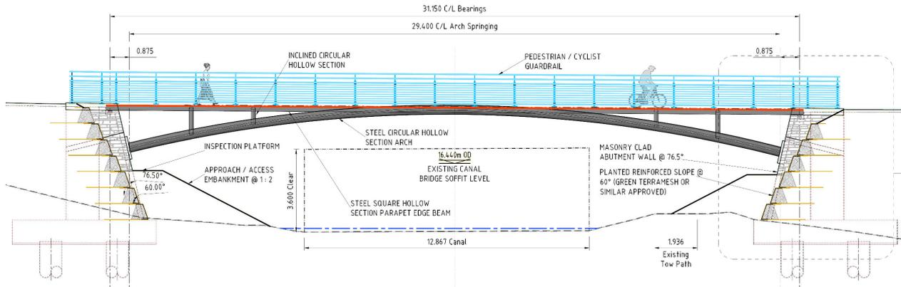
**Figure 4.13: Proposed Span Arrangement of the Shared Use Cycle and Pedestrian Bridge**
