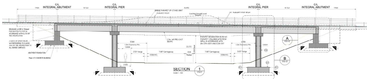
**Figure 4.12: Typical Arrangement of the Overbridges**
