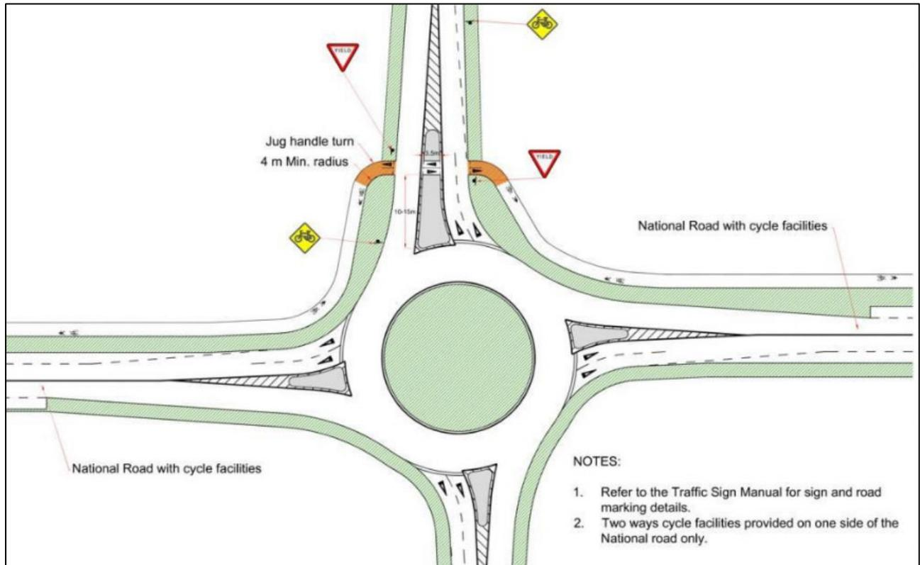
**Figure 4.7: Recommended Arrangement for NMU Crossings at Roundabout Junctions**
