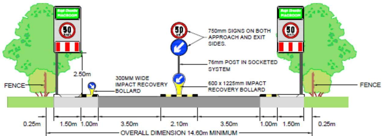
**Figure 4.8: Illustration of Type B Gateway**
