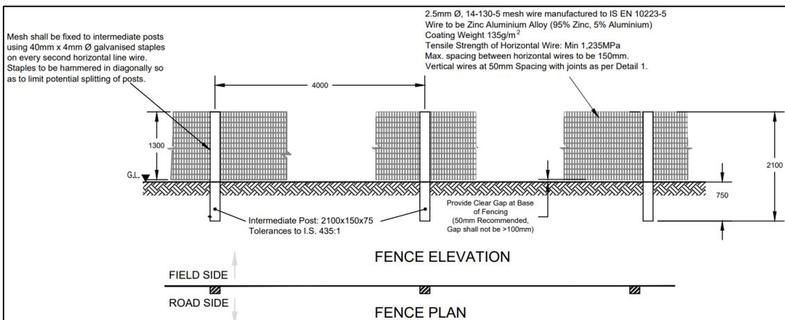
**Figure 4.33: Timber Post and Tension Mesh Fence (Taken From TII CC-SCD-00320)**
